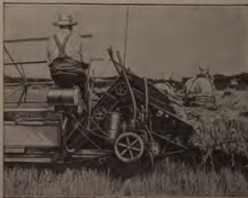
To Make the Operation of a Binder Independent of the Bull Wheel, a Gasoline Motor is Bolted to the Frame. Its Power Drives the Binding Mechanism, Relieving the Bull Wheel of This Duty
